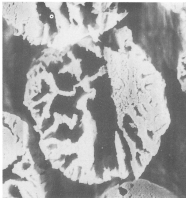
Figure 11 Scanning electron micrograph ( \times 1000 ) of the cross-section for modacrylic fibre of sample P4.
